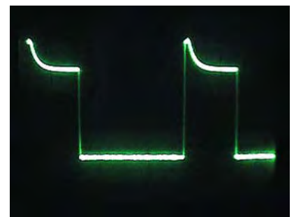
Figure 4. Port loaded with 33 k \Omega .
